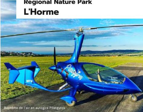
An autogyro flight over Le Pilat. Take a trip up in an ultralight autogyro, and fly over the Massif du Pilat and the Monts du Forez as the fancy takes you... The ultralight autogyro is like a small two-seater helicopter, with the essential difference that it is not propelled by its top rotor, but by a smaller rotor underneath (like a propeller), for a totally safe flight.
